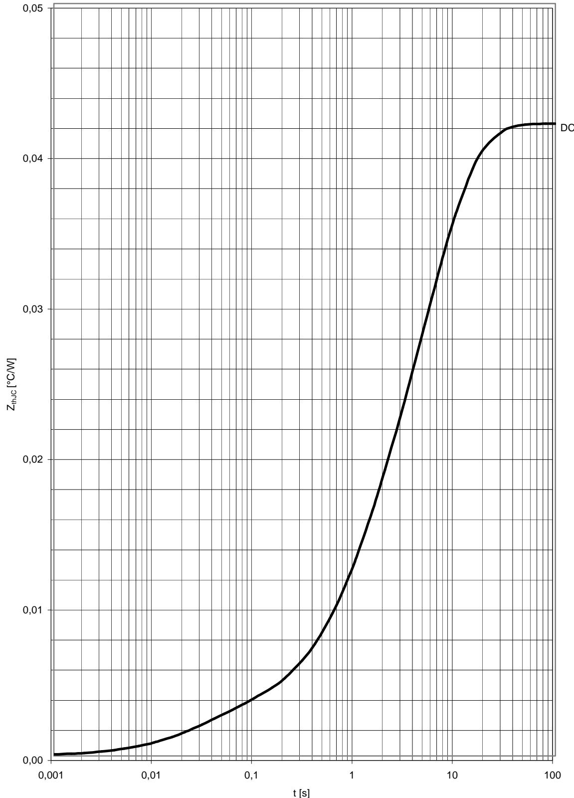
Transienter innerer Wärmewiderstand / Transient thermal impedance  $Z_{thJC} = f(t)$
